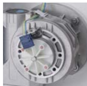
Gear box protection (hall effect)
